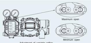
Adjustment of variable orifice
