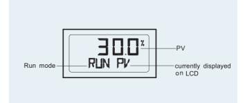
LCD equipped outside of product makes to check the positioner condition in the field directly.
