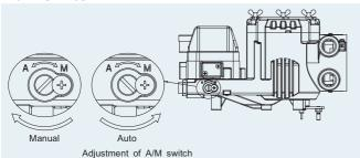
If this switch is set as auto, supply pressure is transmitted to actuator by the operation of YT-2400 and if it is set as manual, supply pressure of air filter regulator is transmitted to actuator regardless of YT-2400.
